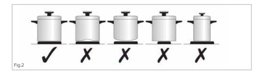
The table below shows the sizes of pan that should be used with each hotplate:
